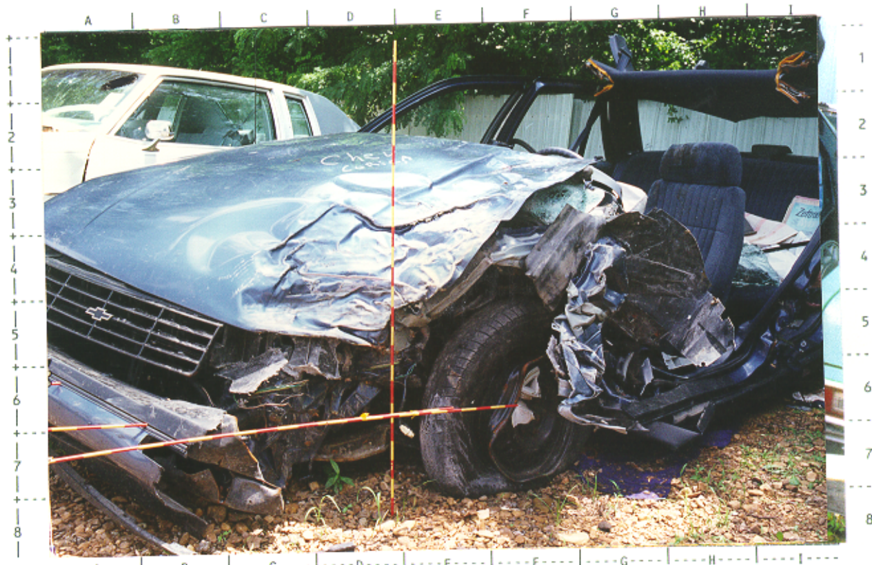
# 33 -- Front left (45 degree angle) view of direct damage to 1991 Chevrolet Corsica; NOTE: peeled-back roof and cut L A- & B-pillars
